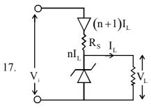
Voltage drop across zener diode is  $\,V_{\scriptscriptstyle L}\,$  so voltage drop across  $\,K_{\scriptscriptstyle S}\,$
