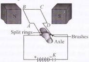
State the direction of movement of sides AB and CD when the key is switched on.
