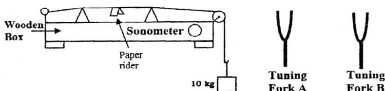
The diagram above shows a wire stretched over a sonometer. Stems of two vibrating tuning forks A and B are touched to the wooden box of the sonometer. It is observed that the paper rider (a small piece of paper folded at the centre) present on the wire flies off when the stem of vibrating tuning fork B is touched to the wooden box but the paper just vibrates when the stem of vibrating tuning fork A is touched to the wooden box.
